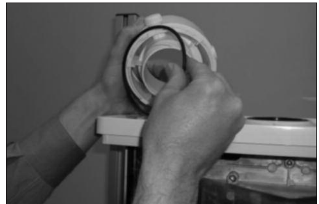
Fig. 6: Installation of O-Ring
